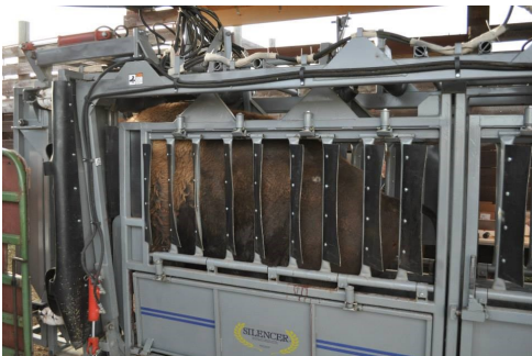
During their examination, bison are held in a hydraulic squeeze chute. This chute keeps the animal from thrashing, which could cause injury to the animal or the staff completing the examination. The bull shown in the squeeze chute was one of the tallest bison to come through. He measured 5'8" at the shoulder. Interestingly, he was not the heaviest. The heaviest bison weighed 1950 pounds.
